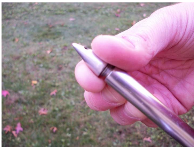
Figure 3: Installation of the soil compaction tester tip. (Photo Credit: Steve Yergeau)
