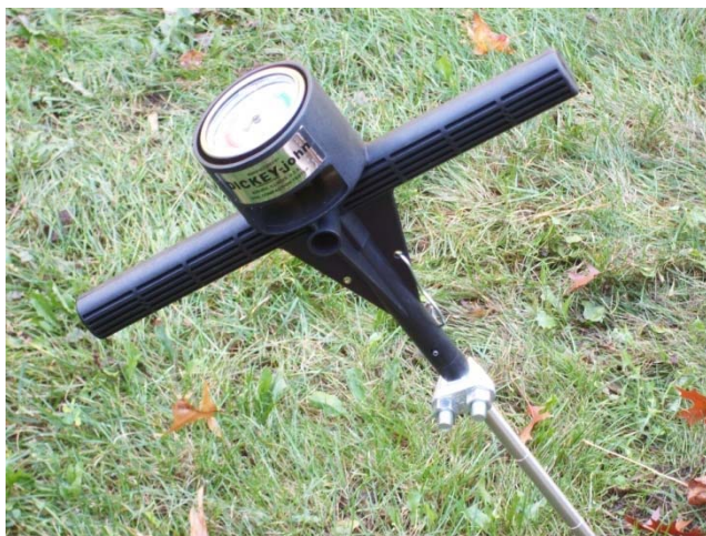
Figure 2: Soil compaction tester with locking ring in place. (Photo Credit: Steve Yergeau)
