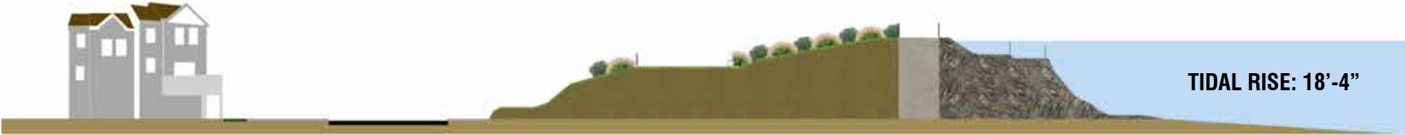
Flood Protection Diagram B: Projected Storm Surge In 2050 *Sea Level Rise: 4" The Seawall Successfully Protects Union Beach From Storm Surges Bigger Than Hurricane Sandy
