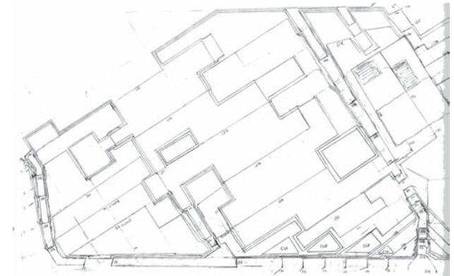
Figure 16. A test grading plan of the central space with a 1% slope through the central space draining toward the meadow.
