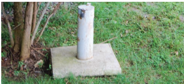
Figure 4. Monitoring wells like this one are found around the border of the site, protruding 18 inches above grade.
