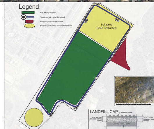
Figure 2. Cap and Contamination Analysis Map
