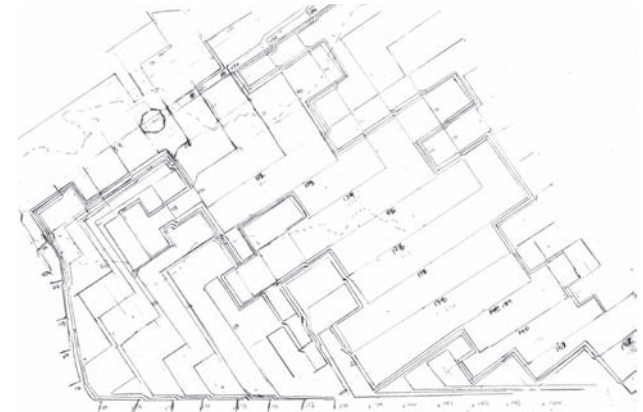
Figure 17. A test grading plan of the central space with a 2% slope through the central space draining toward the meadow.
