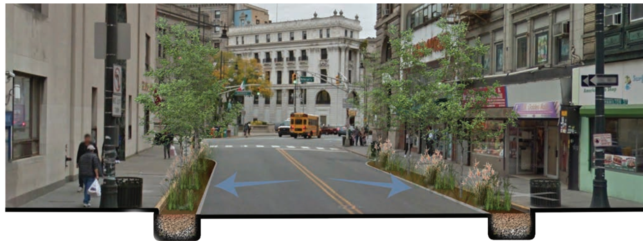
A section perspective of Market Street in Paterson New Jersey. These 6 foot wide "Roadside Bioswales" can be implemented on medium to large streets to hold and retain stormwater runoff and lessen the amount of rainwater that ends up in Combined Sewer Systems
