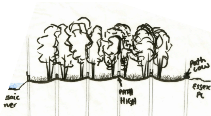
Concept drawing of a section view showing the relationship between detention basins and walking paths are wave-like.
