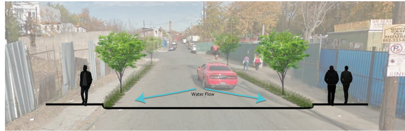
A section perspective of Presidential Boulevard in Paterson New Jersey. These 2 foot wide "Green Gutters" can be implemented on more narrow streets to maximize the storm water retention within a small area
