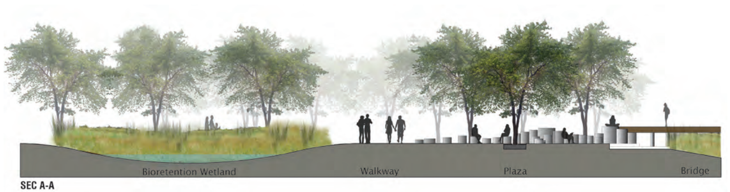
figure 12: Section through Plaza and Wetland
