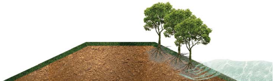
Figure 3.3.2: Berm Seepage From Tree Roots
