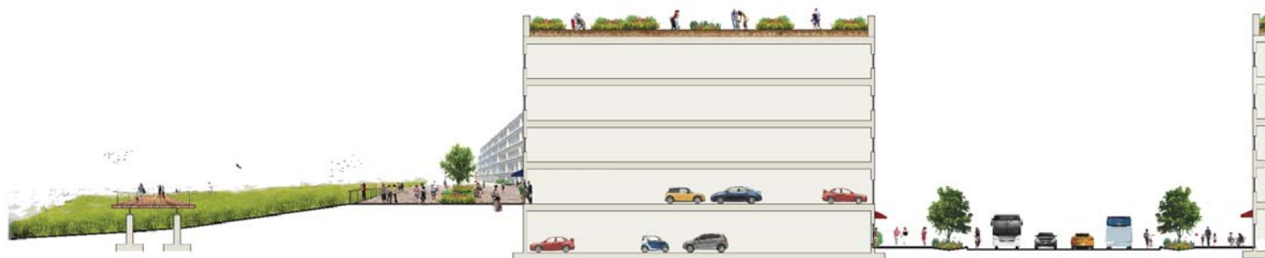
Fig. 4.5.2.5 Section of Bergen Turnpike illustrating the wetland park, pedestrian promenade on berm, parking concept, green roofs, and streetscape improvements.
