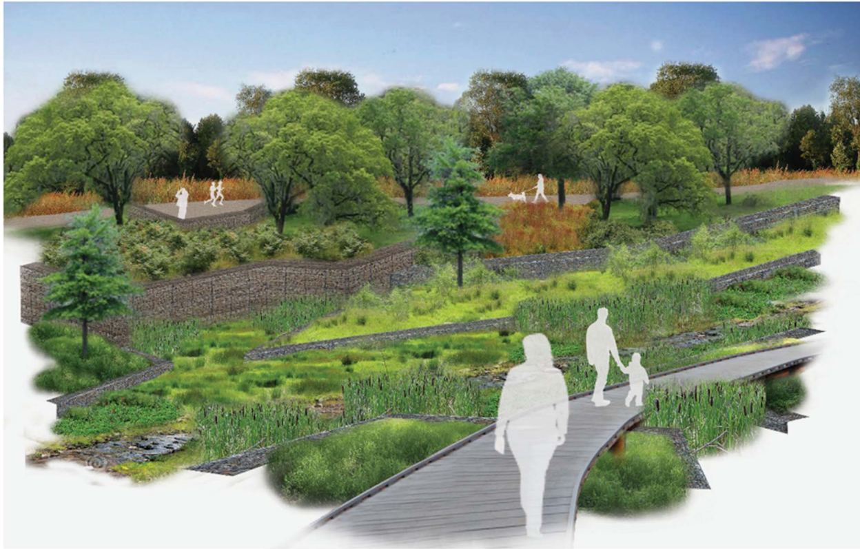
Figure 7. Rendering of the transition area between the proposed capped Somerville Landfill and the existing wetland. The proposed enhanced wetlands increase stormwater retention while serving as points of public access.
