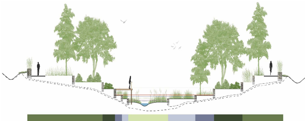
Figure 8. Typical cross-section indicating elevations needed to capture various storm events, creating both facultative and obligate hydric planting zones. In addition, the approximate depth of fill required to develop shrub and forest guild assemblages is indicated.
