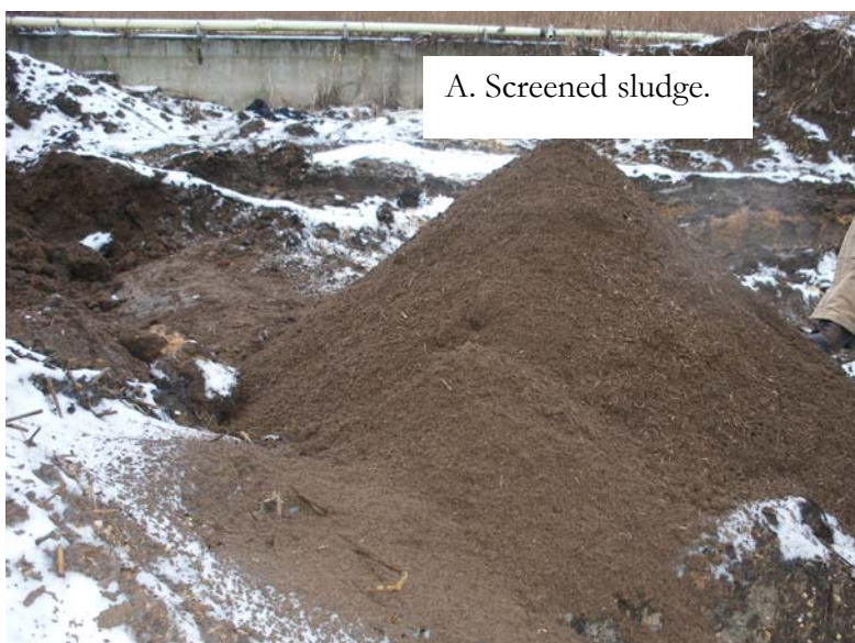
Fig. 11. WMUA sludge pre (b) and post (a) screening with McCloskey 412 trommel screener.
