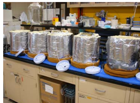
Fig. 1. Insulated and aerated bench top compost experiment.
