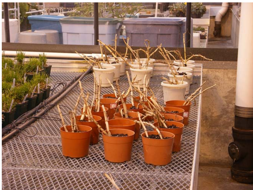
Fig. 8. Phragmites rhizomes recovered from large WMUA compost pile after interior pile temperature reached 55 degrees C.
