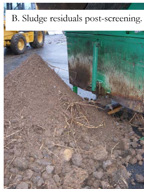
Fig. 11. WMUA sludge pre (b) and post (a) screening with McCloskey 412 trommel screener.
