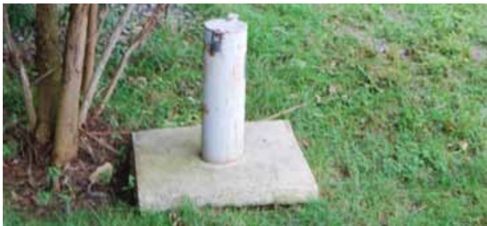
Figure 7. Monitoring wells like this one are found around the border of the site, protruding 18 inches above grade.
