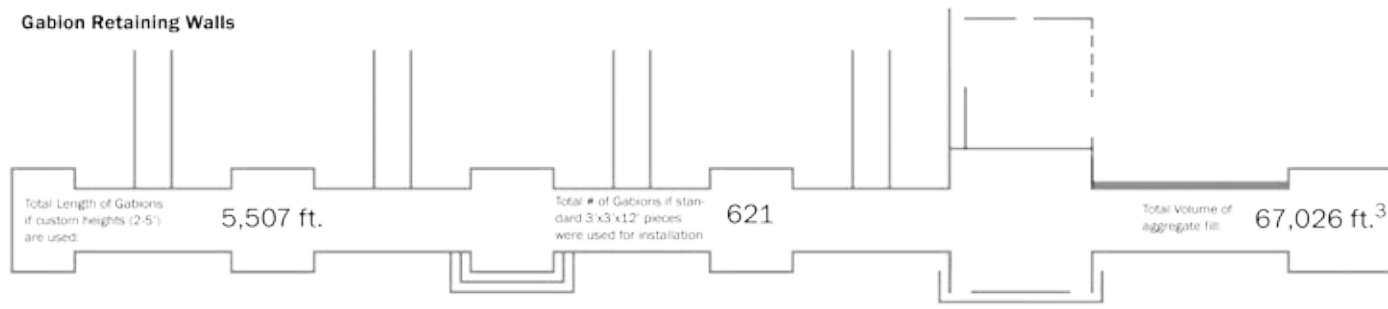
Figure 79. Diagram of gabion use at Voorhees Environmental Park with approximation of casing length and fill volume.
