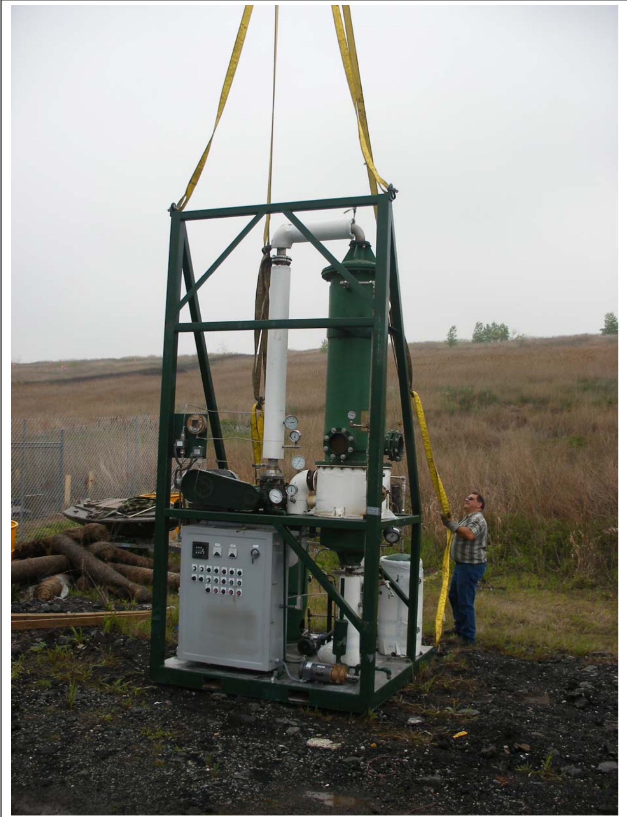
Fig. 12. Field pilot evaporation system constructed by Rosenblad Design Group, Inc.
