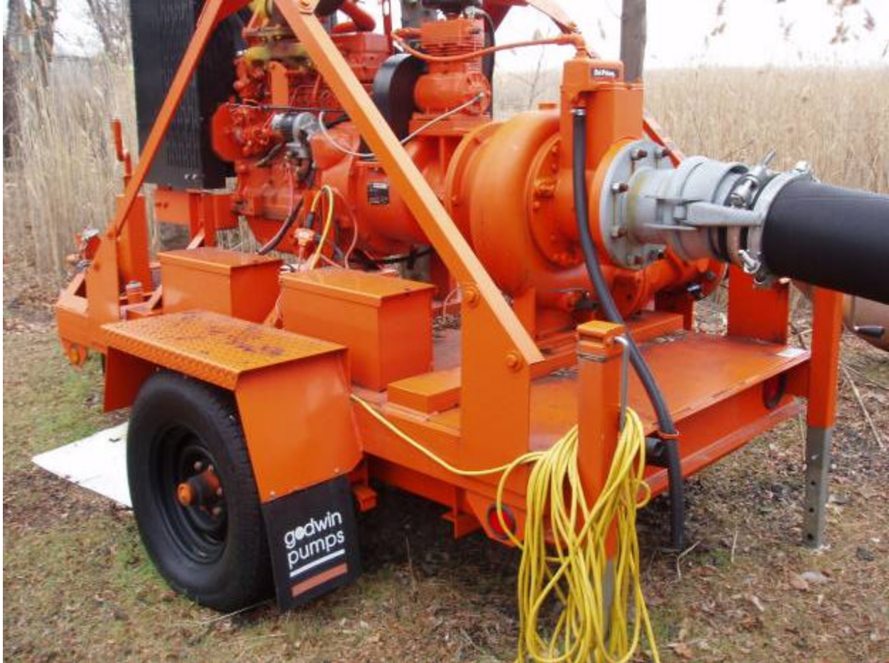
Photo 3 Description: Godwin diesel back-up pump system
