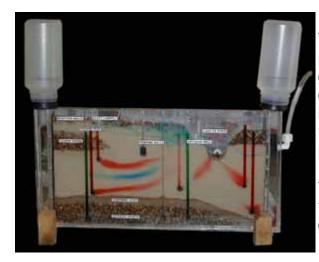
The groundwater model is a plexiglass tank filled with sand, gravel, and clay to represent a slice of the earth. The model simulates how water and contaminants move through different aquifers allowing people to "see" groundwater.
