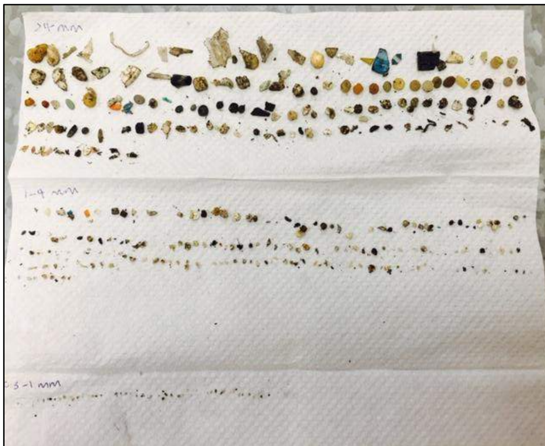
Figure 10. Plastics separated into size categories three size classes (0.355-0.999 mm, 1.00-4.749 mm, and >4.75 mm) after counting.
