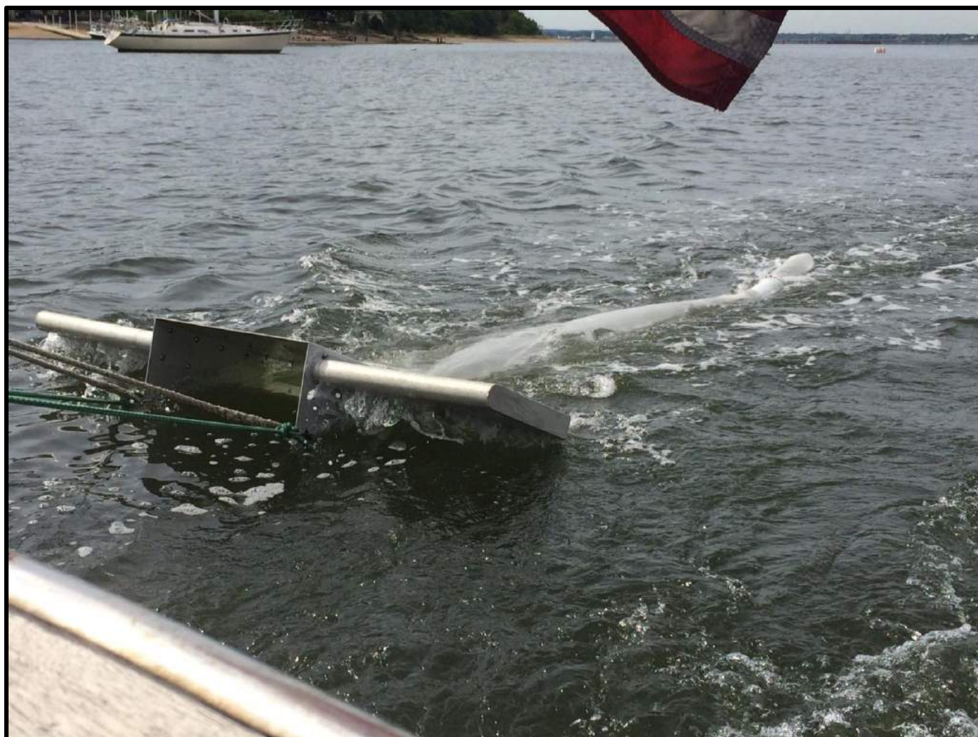
Figure 1. Manta trawl net used for plastic collection along Staten Island, NY shore
