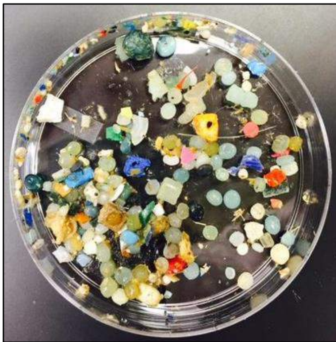
Figure 9. Plastic sample collected from Newark Bay exhibited pre-production pellets (nurdles) and microplastic fragments.
