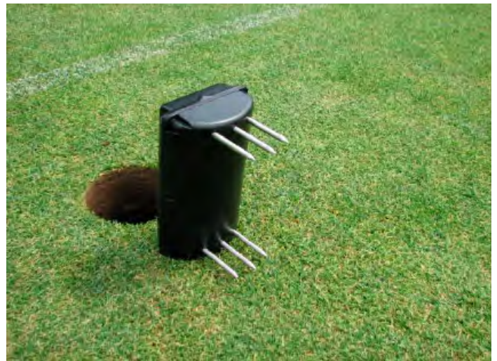
Figure 25. Moisture meters as part of an integrated irrigation management system (Courtesy of John J. Genovesi/Maidstone Club 11 ).
