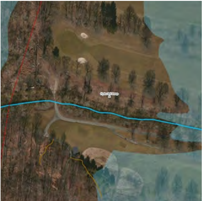
Figure 22-23. Without adequate stream buffers, shallow concentrated flow running into water bodies creates the potential for stream degradation at Rockleigh Golf Course (Courtesy of Biohabitats).
