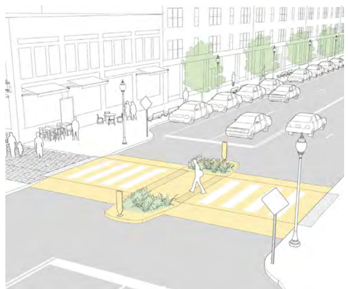
Figure 9. Raised crosswalk for safe passage (Courtesy of NACTO).
