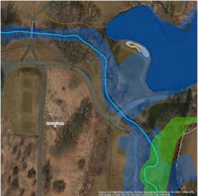
Figure 20. Limited vegetative buffers do not provide enough root protection, increasing the risk of stream bank erosion (Courtesy of Biohabitats).
