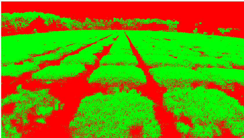
Figure 2. Using machine learning and segmentation analysis, the robot is trained to recognize vegetation areas (green) that should not be traveled on and potential paths (red) that can be traveled on. Additionally, breaks between vegetation segments, combined with GPS coordination, will denote specific plot locations where measurements will be taken.
