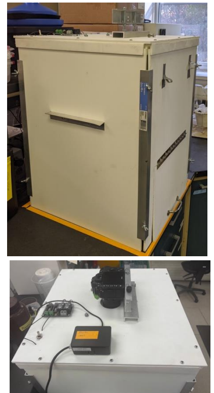
Figure 2. The BerryBox system includes (top) a lightbox and (bottom) a microcomputer to capture images using a DSLR camera.
