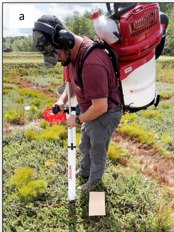
Picture 3. Cranberry research plots harvesting operations with the Cifarelli V1200E vacuum harvester . a) vacuum sucking of the fruits; b) lever to open the tank containing harvested berries; c) berries unloading; d) berries harvested with the Cifarelli V1200E vacuum harvester
