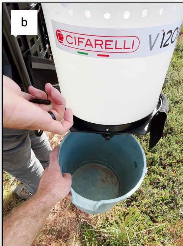
Picture 3. Cranberry research plots harvesting operations with the Cifarelli V1200E vacuum harvester . a) vacuum sucking of the fruits; b) lever to open the tank containing harvested berries; c) berries unloading; d) berries harvested with the Cifarelli V1200E vacuum harvester
