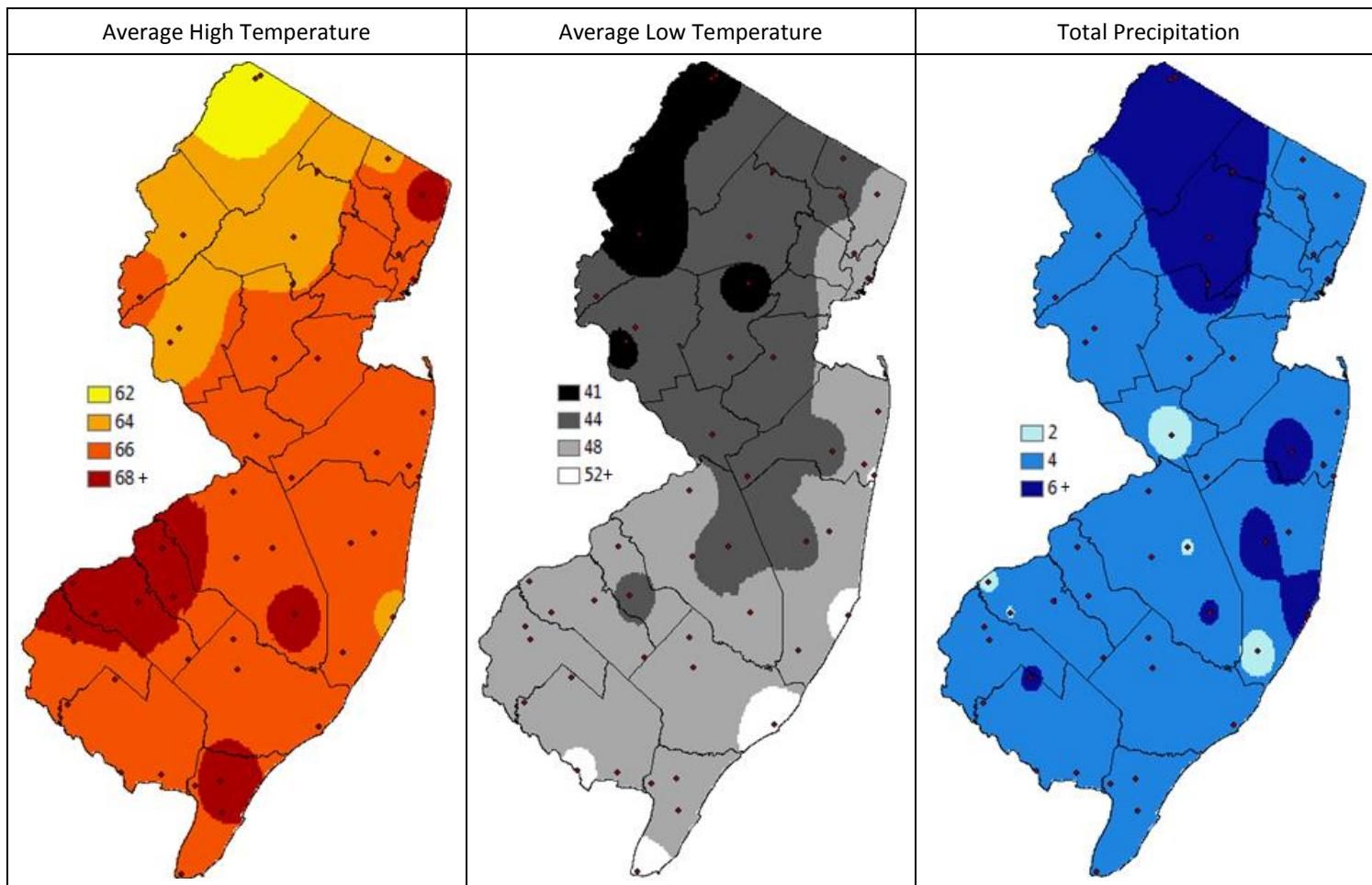
The three figures show the interpolation of average maximum (°F) and minimum temperature (°F) and total precipitation (inches) for 30 days prior to 9 November 2017 in New Jersey. Data points are from about 54 weather stations maintained through the New Jersey Weather & Climate Network and the State Climatologist. Interpolation between points was performed using ArcMap 10.1.
