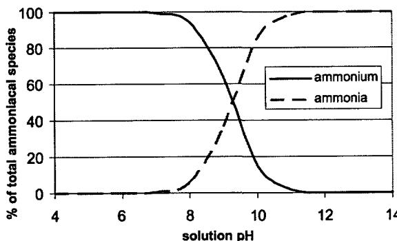
**FIGURE 1.** Dominant form of ammoniacal nitrogen in solution at 25°C at various pH levels.
